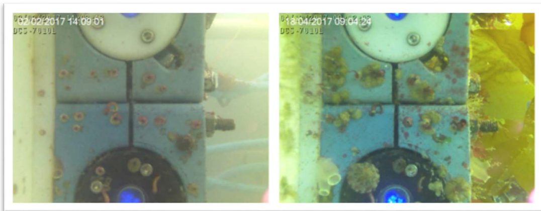
Figure 14: HD camera snapshots showing no biofouling effect on the images. (Photos: Ifremer)
