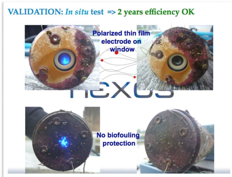
Figure 10: SnO 2 conductive layer biofouling protection efficiency test on fluorimeter sensors (Ifremer in situ testing bench).
