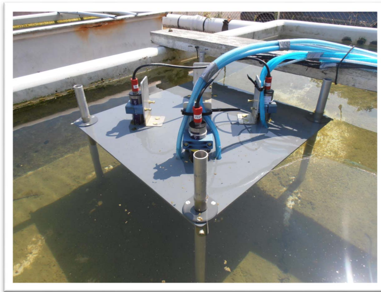
Figure 9: In situ testing bench for biofouling protection efficiency. (Photo: Ifremer - L.Delauney).
