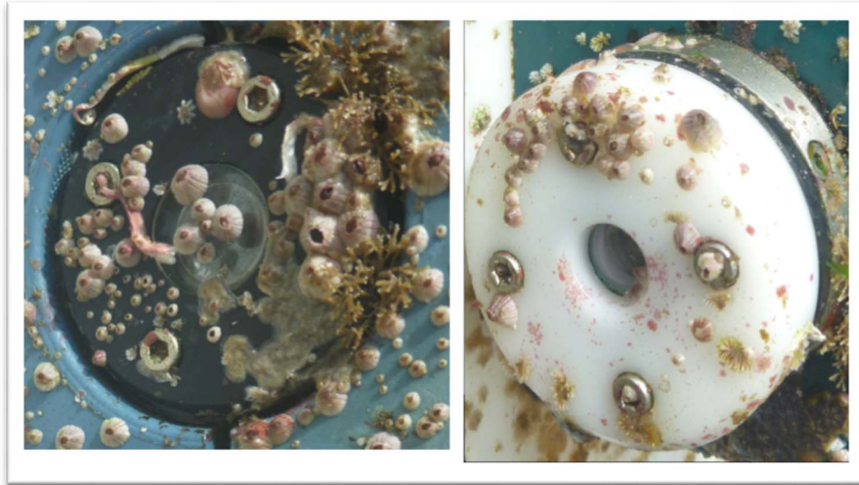
Figure 13: Sensors after 6 months of exposure to natural seawater. Left : unprotected sensor ; Right : SnO 2 protected sensor.
