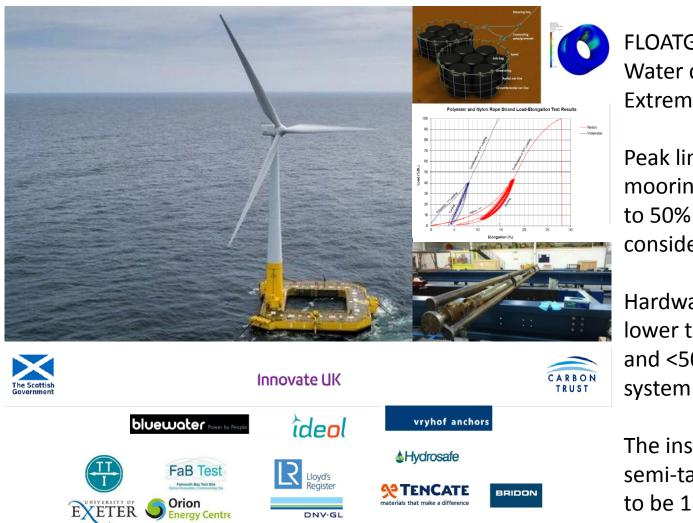
FLOATGEN displacement ~6000T Water depth = 32m Extreme design Hs = 9m
