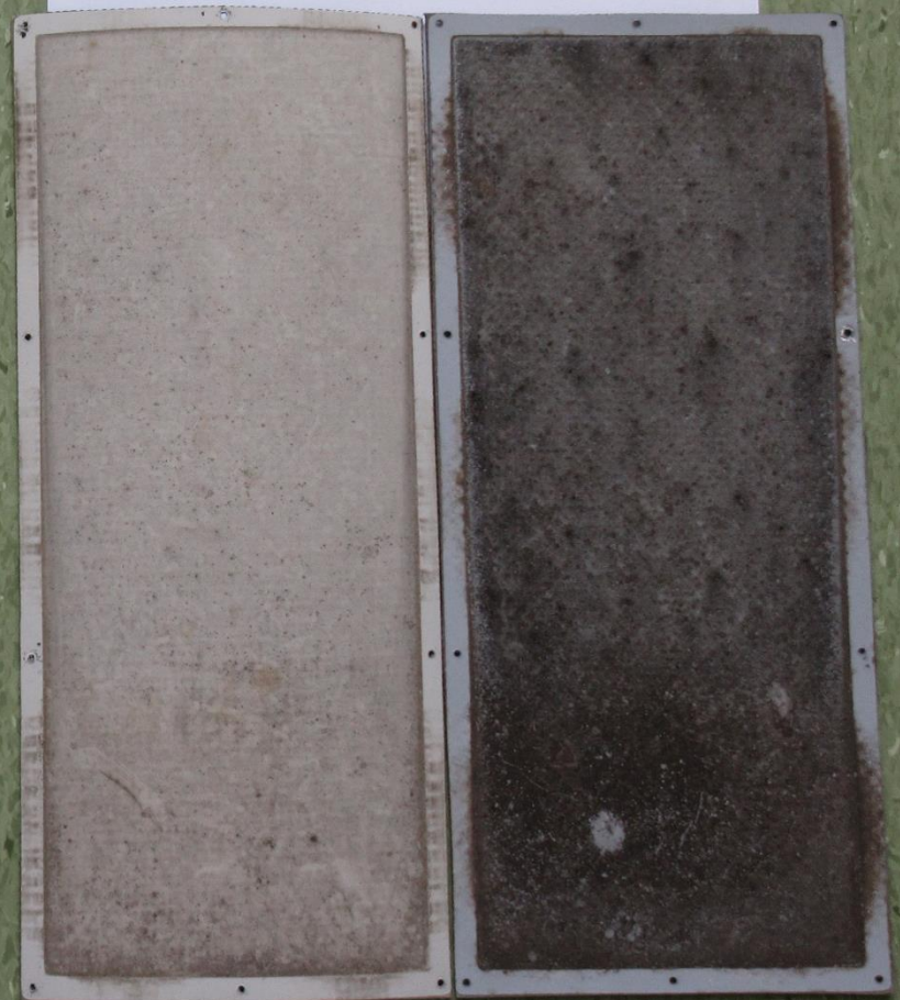
Airborne pollutions demonstrated on roofing materials tested together with PP
