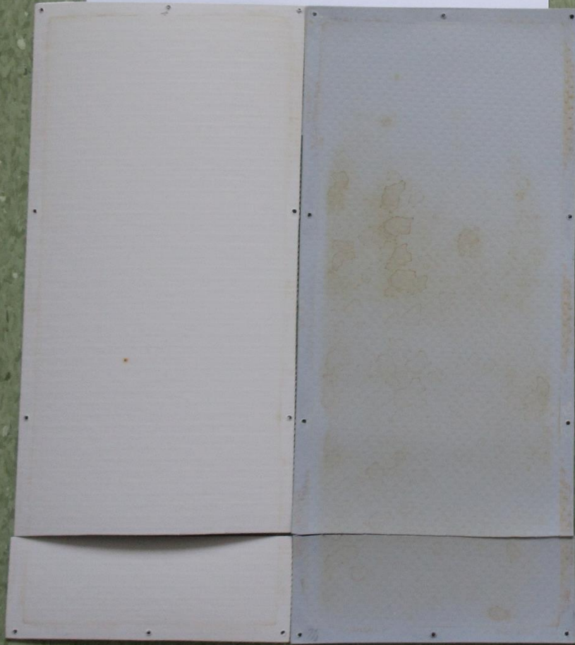
Airborne pollutions demonstrated on roofing materials tested together with PP
