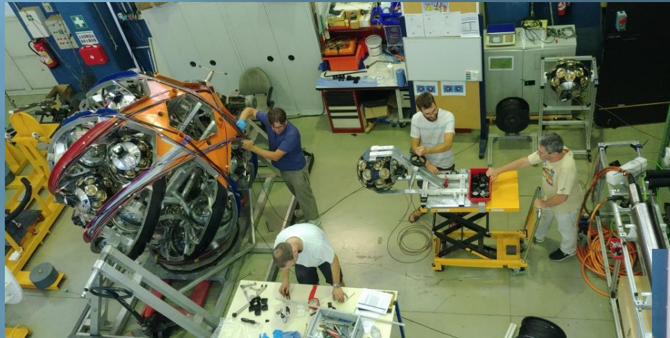
Installation of the DU on the LOM
