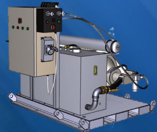
Hydraulic power unit
