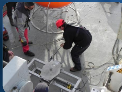
Cable in the return pulley
