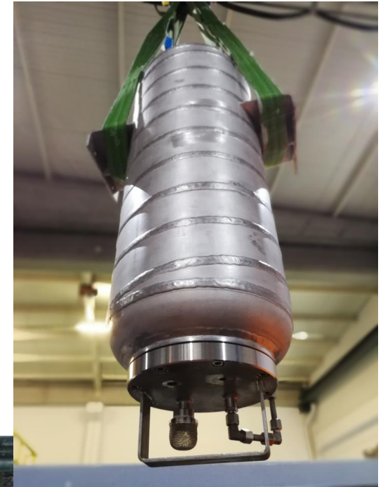
Integrated pressure vessel (water + hydraulics/electronics)
